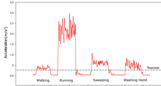
Figure 4: Standard deviation threshold for trunk accelerometer signals
